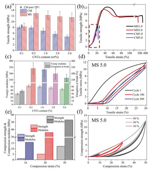
Fig. 4 (a) Tensile strength of the pure TPU prepared by compression molding, CM and MS samples with various CNT contents; (b) typical tensile stress–strain curves of the MS and CM samples with 1.0 wt% and 5.0 wt% CNT; (c) elongation at break and tensile modulus; (d) cyclic stretching-recovery curves of  $MS_{5.0}$ ; (e) compression strength and modulus; (f) cyclic stress–strain curves of  $MS_{5.0}$  at various compression strains.
