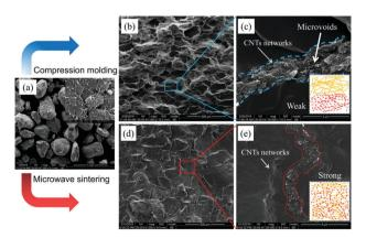
**Fig. 2** SEM images of (a) TPU/CNT complex granules (inset shows the magnified image); (b) the fractured surface of the  $CM_{5.0}$  composite; (c) the magnified SEM image of (b); (d) the fractured surface of the  $MS_{5.0}$  composite; (e) the magnified SEM image of (d).
