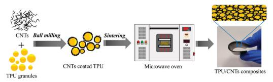
Fig. 1 Schematic of procedure for fabricating TPU/CNT composites via MS.
