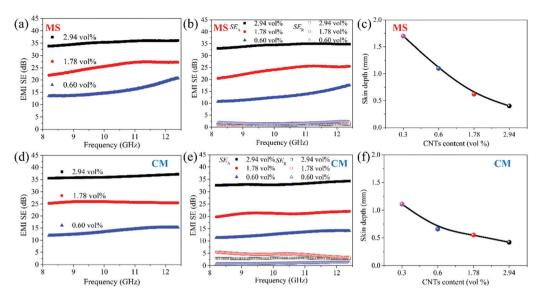
Fig. 6 (a and b)  $SE_T$ ,  $SE_A$ , and  $SE_R$  for the MS samples; (c) skin depth of MS vs. CNT volume content; (d and e)  $SE_T$ ,  $SE_A$ , and  $SE_R$  for the CM samples; (f) skin depth of CM with different CNT volume contents. (The thickness of the sample is 2.0 mm.)
